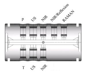
Fig. 1: Combined cell for inline monitoring containing Raman and NIR transmission and/or reflection probes, pressure (p), temperature (T) and ultrasonic transducers (US).
